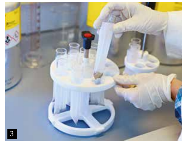
When the FibreBags are inserted into the sample carousel, they are automatically clamped firmly in place.
