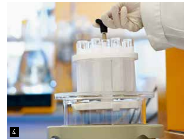
The removable handle makes it easier to insert and remove the sample carousel.
