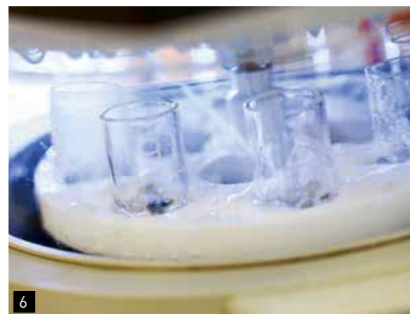
The rotating sample carousel ensures optimum bathing of the sample. The rotation is generated by the jet of detergent.
